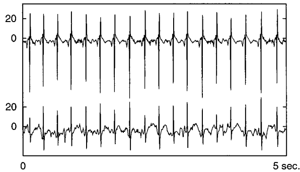
FIG. 8. Top: original fetal component included in the series shown in Fig. 1. Bottom: reconstructed fetal component after nonlinear noise reduction. Although the amplitude of the fetal QRS complex is reduced in the reconstruction, at least the heart rate can be determined reliably.
